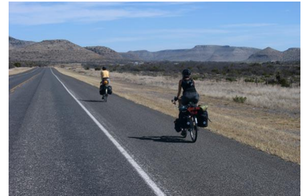
WHILE A SHARED USE PATH IS PREFERRED IN ALL CASES, THIS PHOTO SHOWS A LOW MOTOR VEHICLE VOLUME CONTEXT WHERE A SHOULDER CAN BE APPROPRIATE (PHOTO COURTESY TxDOT)
