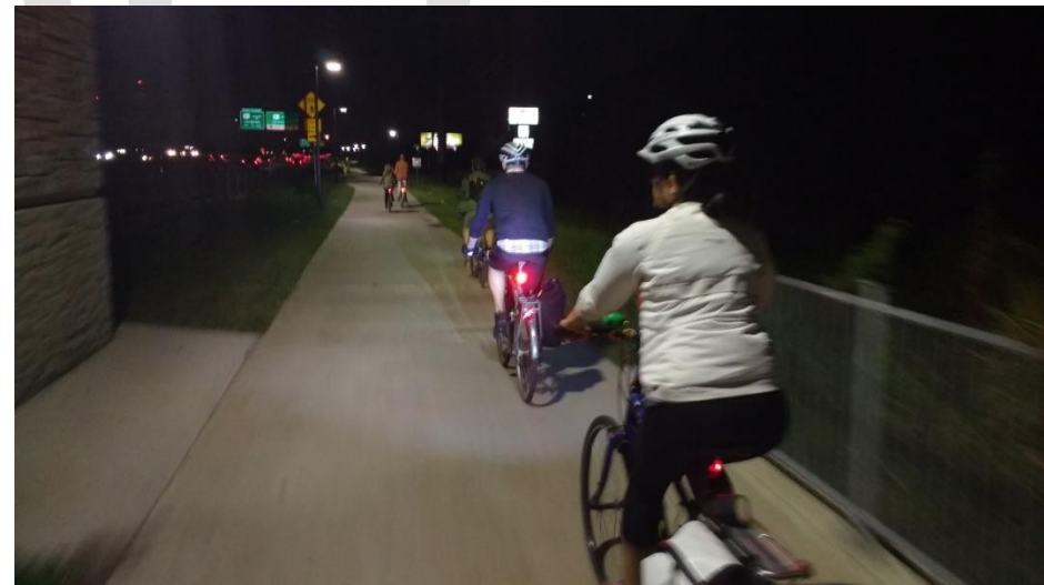
LIGHTING ALONG THE HW 71 SHARED USE PATH IMPROVES VISABILITY AND COMFORT OF THE PATH, IMPROVES SAFETY, AND REDUCES HEADLIGHT GLARE THAT AFFECTS NIGHT VISION
