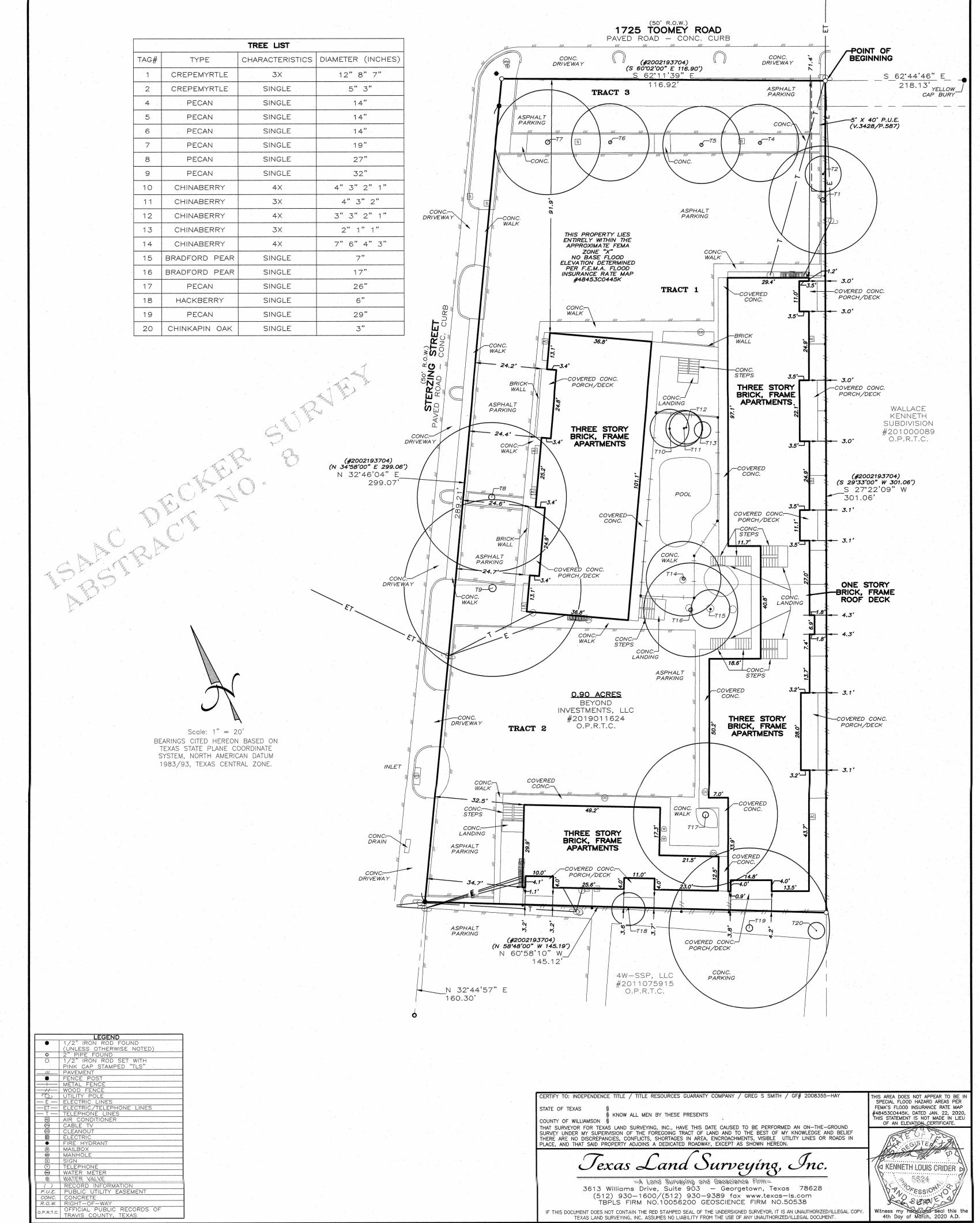
Scale: 1" = 20'BEARINGS CITED HEREON BASED ON TEXAS STATE PLANE COORDINATE SYSTEM, NORTH AMERICAN DATUM 1983/93, TEXAS CENTRAL ZONE.
