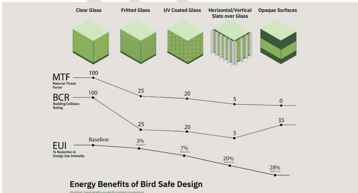
Figure 9. 5Reduction in energy use when compared across five bird friendly material performance conditions. (Pawar, 2024).
