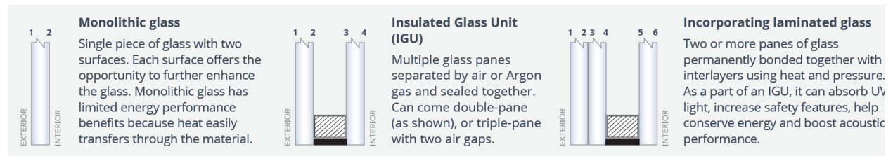
Figure 4 This diagram shows the layers of glass and corresponding surface numbers. Best practice is for bird deterrence measures to be on surface 1 of the glass. Image from Guardian Glass
