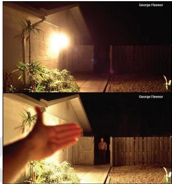
Figure 10. 6The blinding glare from an unshielded light makes the figure in the background invisible to the viewer. Photo credit George Fleenor
