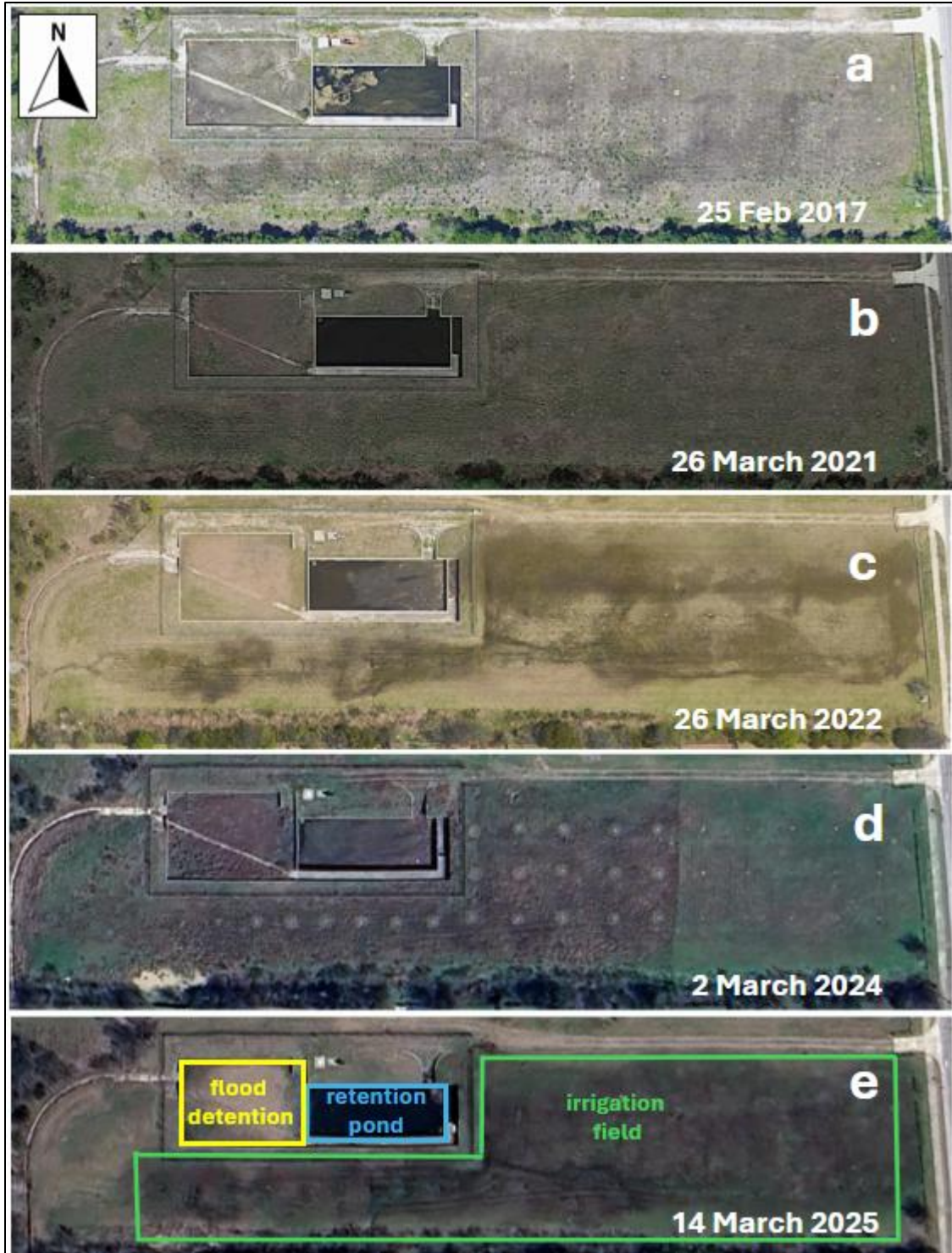
Figure 8 – West Gate R/I pond system typical images selected from the 26 Google Earth aerial photos from 2012-2025. Most (85%) of the available images show the retention basin to be either completely inundated (a, b, e) or partially inundated (c) substantiating the observations of inspection staff that the pump/irrigation system is chronically clogged. Note accumulation of algae in stagnant inundation (a), heterogeneous saturation/standing water around some sprinkler heads (c, e), and organization of surface water that flows to the west (bottom left corner) and has been observed as off-site runoff circumventing treatment (c, d). See Appendix A for a table listing antecedent rainfall and basin status corresponding to available aerial imagery.
