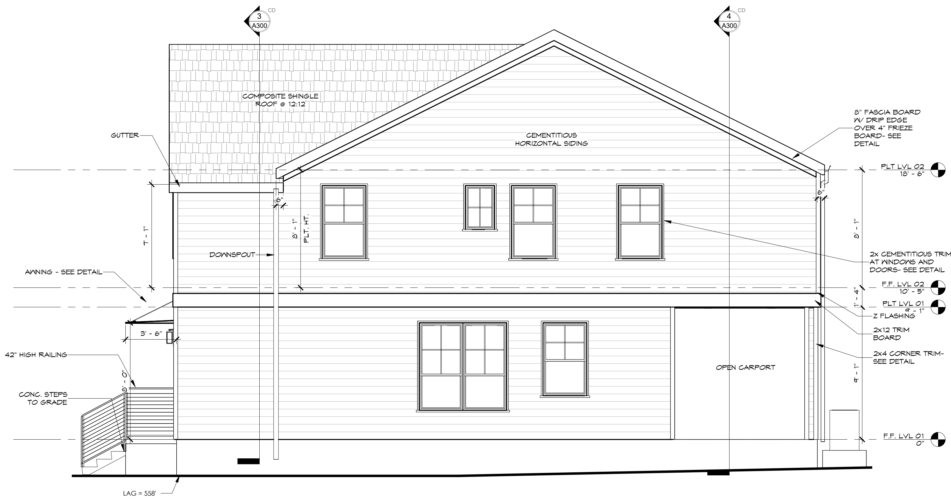
4 BUILDING 1 RIGHT ELEVATION 1/4" = 1'-0" (22x34) 1/8" = 1'-0" (11x17)
